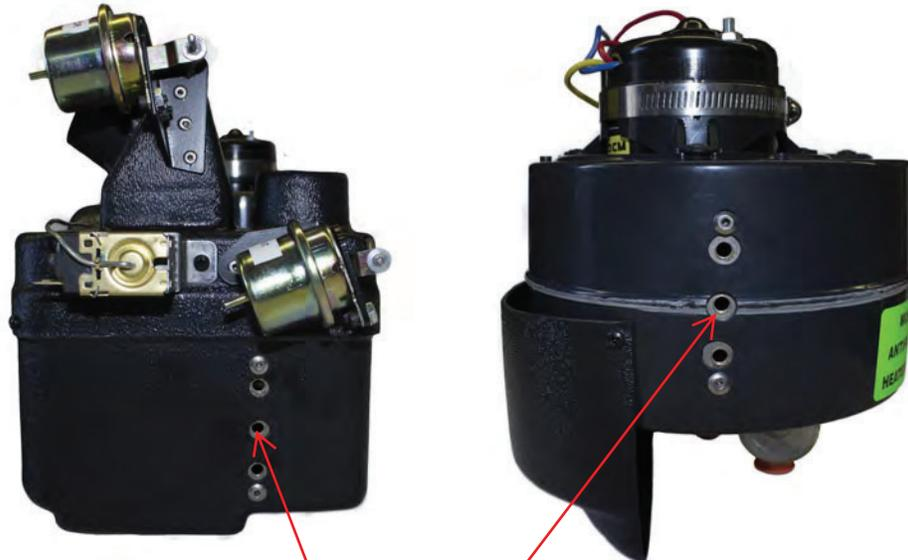
“L” Brackets attach to the sides of the unit. The holes are for adjustment, only one hole is necessary for mounting.
