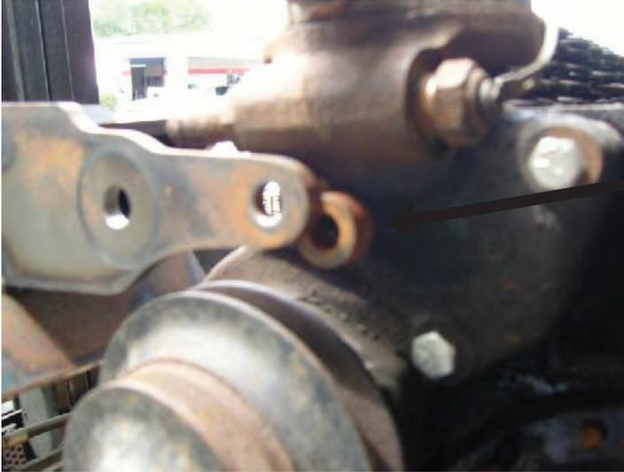
Use the 1/8" water pump spacer between the bracket and the water pump
