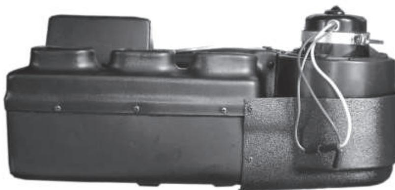
This is how the ID260 / 265 will sit in the vehicle. The right side has a hose cover below the blower motor housing. This is the view of the unit if you were sitting in the passenger seat.
