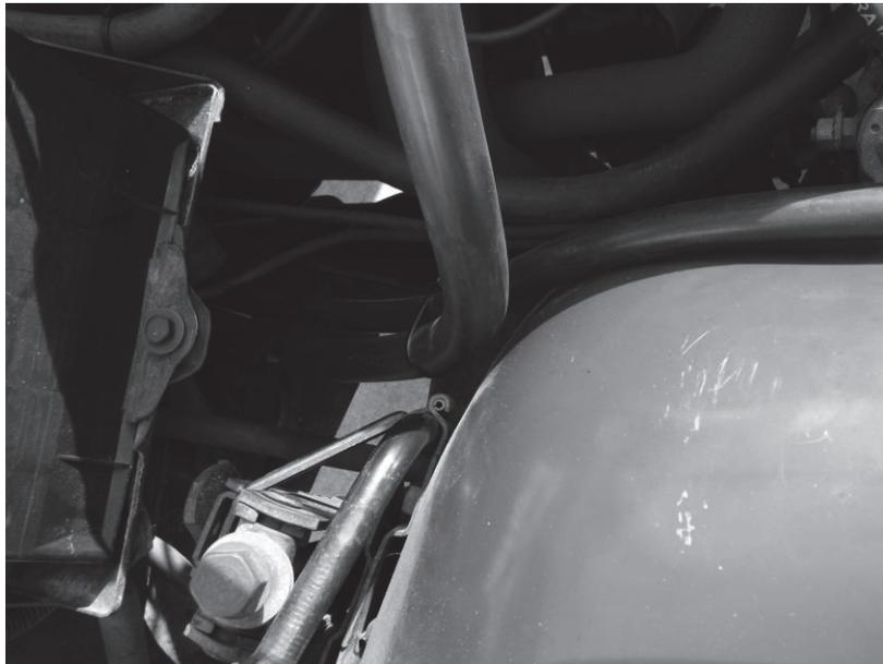
Make sure the hoses do not rub any metal. Securing them with tie straps is recommended.
