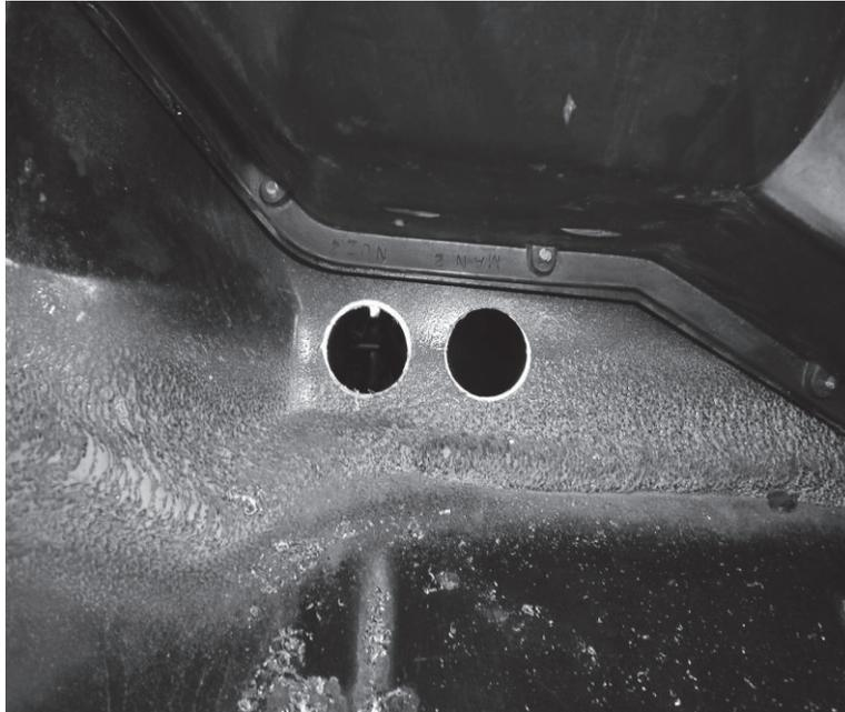
7. Insert the two rubber grommets at this time. Lube may be needed to feed the larger a/c line through the grommet.
