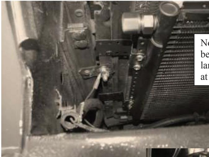
Notice the condenser straps bent into a Z for fitment. The large fitting of the condenser is at the top.
